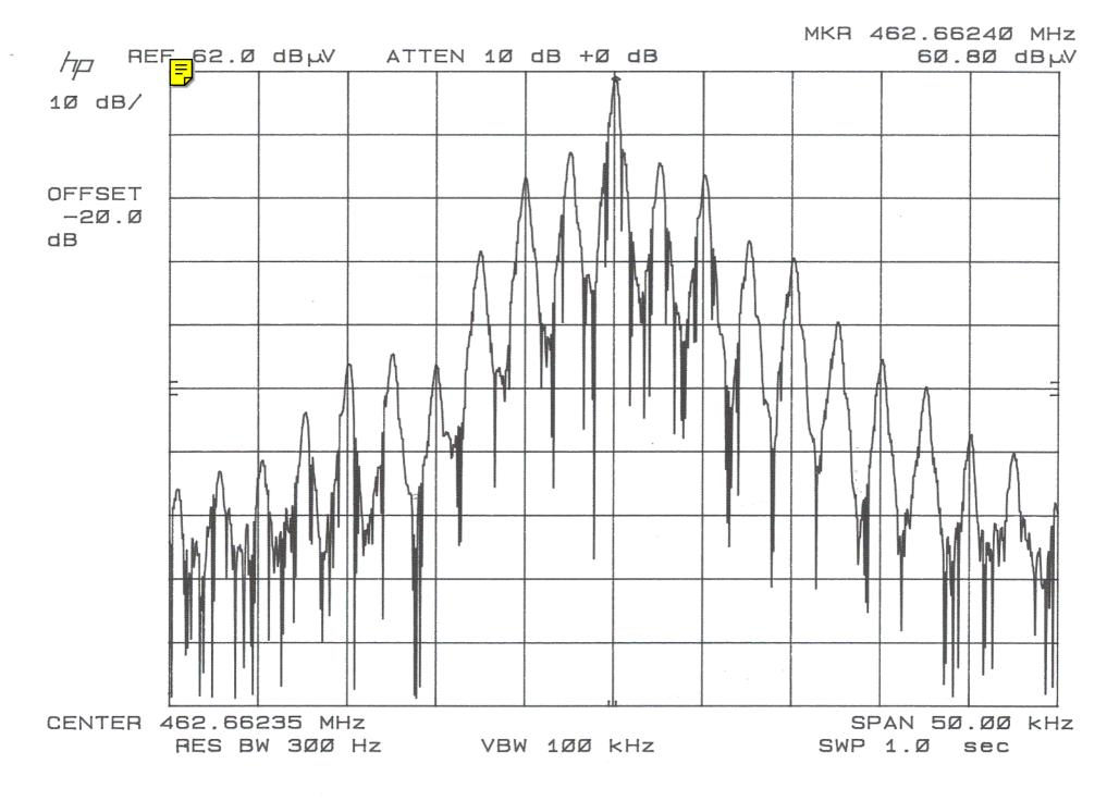
2.1051 Spurious emissions at antenna terminals(conducted): The following data shows the level of conducted spurious responses at the antenna terminal. The test procedure used was TIA/EIA 603 S2.2.13 with the exception that the emissions were recorded in dBc. The spectrum was scanned from 0.4 to at least the 10th harmonic of the fundamental.
