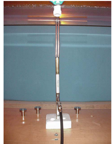
450 MHz Dipole Setup
