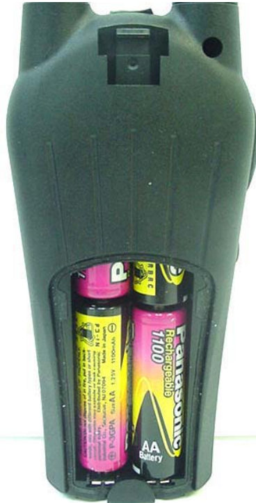
DUT with NiCd AA Batteries
