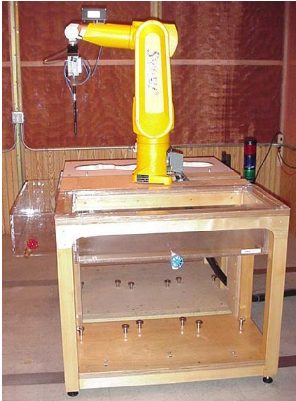
DASY4 SAR Measurement System with validation phantom
