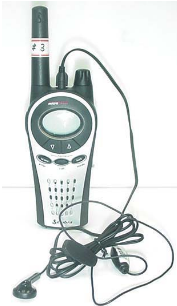
DUT with Earbud/Lapel-Microphone accessory (P/N: GA-EBM2)
