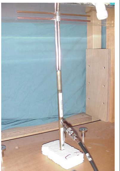
450 MHz Validation Dipole Setup
