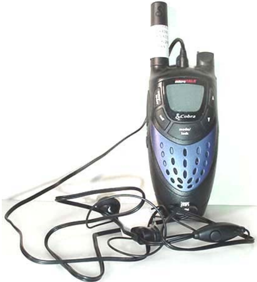
DUT with Ear-bud/Lapel-Microphone Audio Accessory
