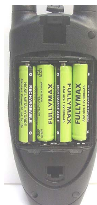
DUT with NiMH AAA Batteries
