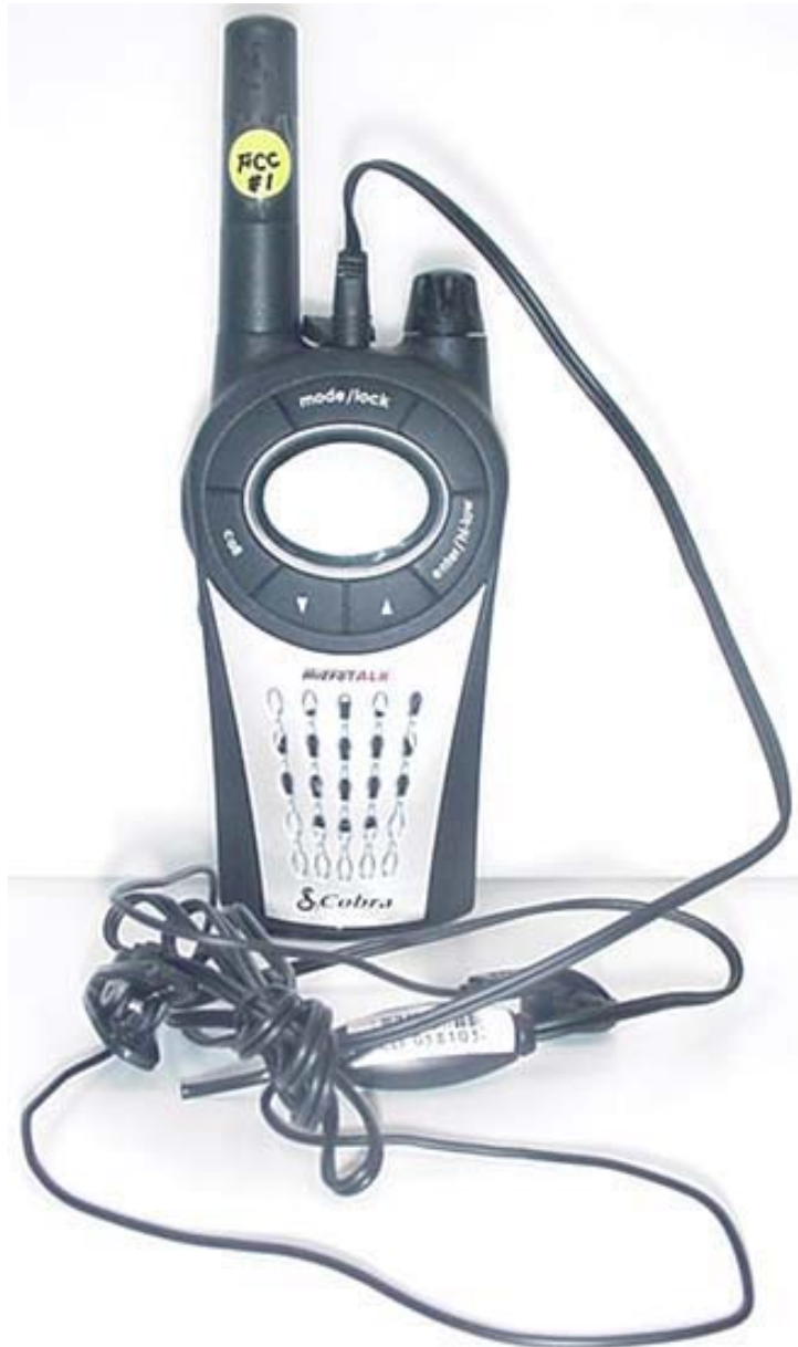
DUT with Earbud/Lapel-Microphone accessory (P/N: GA-EBM2)
