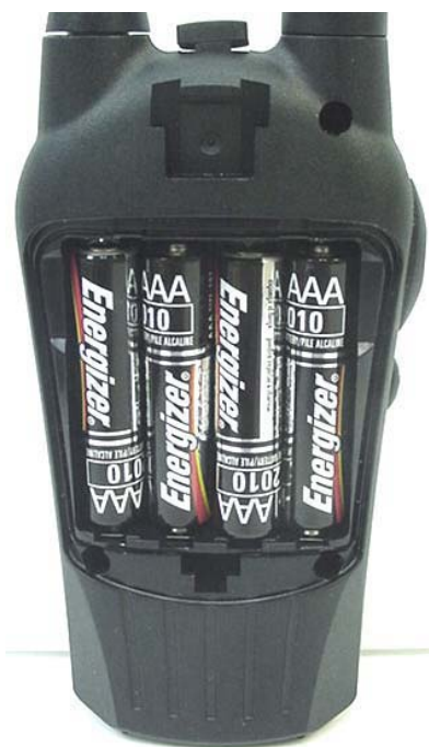
DUT with Energizer E92 AAA Alkaline Batteries
