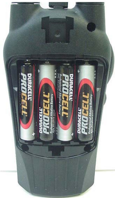
DUT with Duracell Procell AAA Alkaline Batteries
