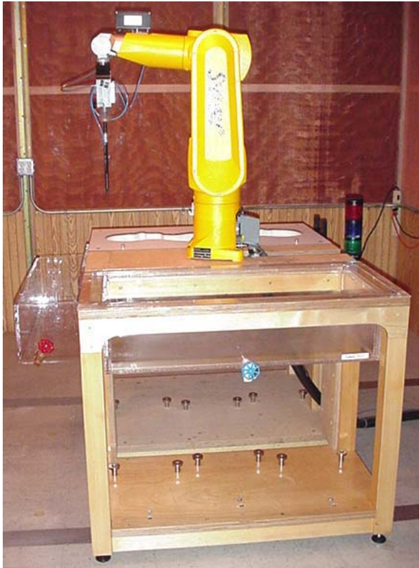
DASY4 SAR Measurement System with validation phantom
