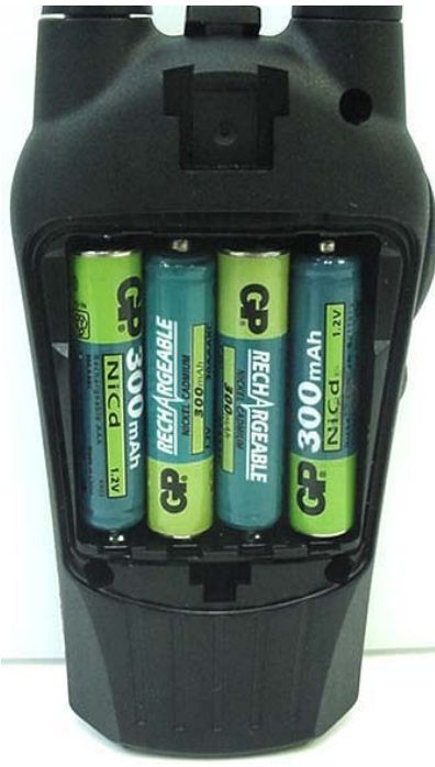
DUT with NiCd AAA Batteries
