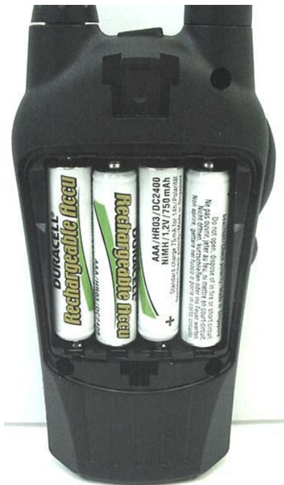
DUT with NiMH AAA Batteries
