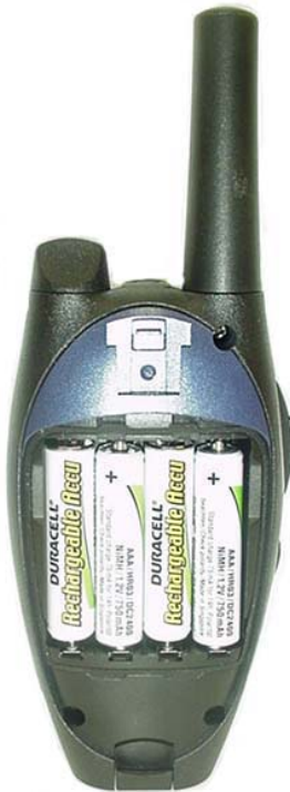
DUT with NiMH Batteries
