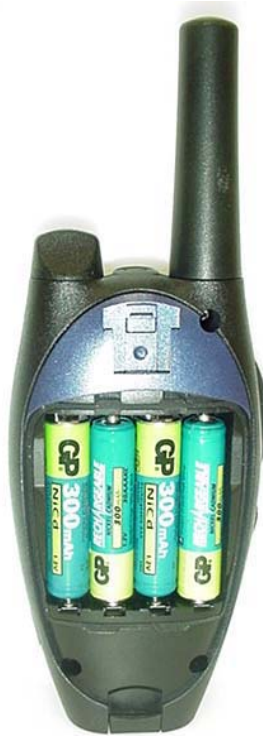
DUT with NiCd Batteries
