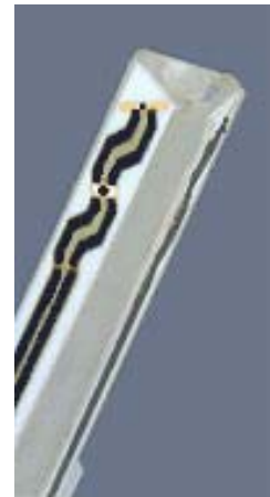
ET3DV6 E-Field Probe
