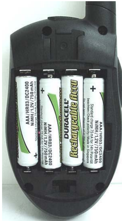
DUT with NiMH AAA Batteries
