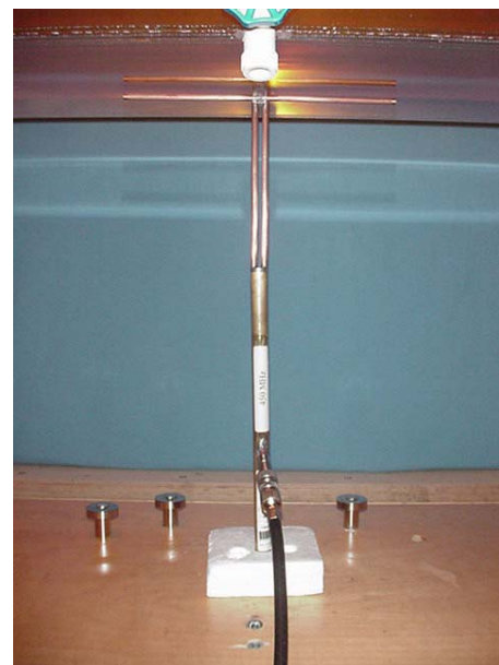
450 MHz Dipole Setup
