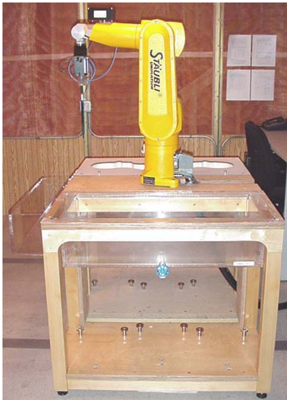
DASY4 SAR Measurement System with validation phantom
