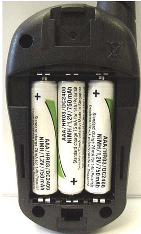
DUT with NiMH AAA Batteries
