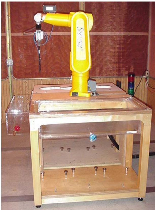
DASY4 SAR Measurement System with validation phantom
