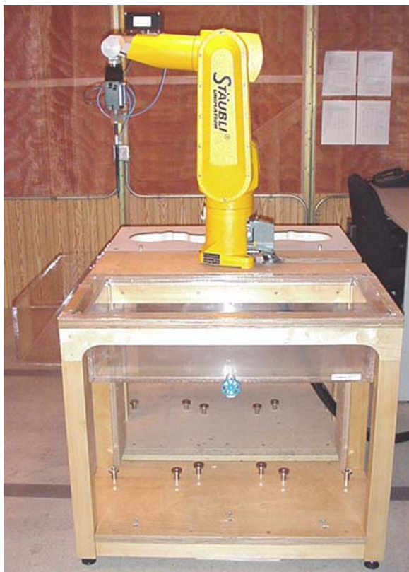
DASY4 SAR Measurement System with validation phantom
