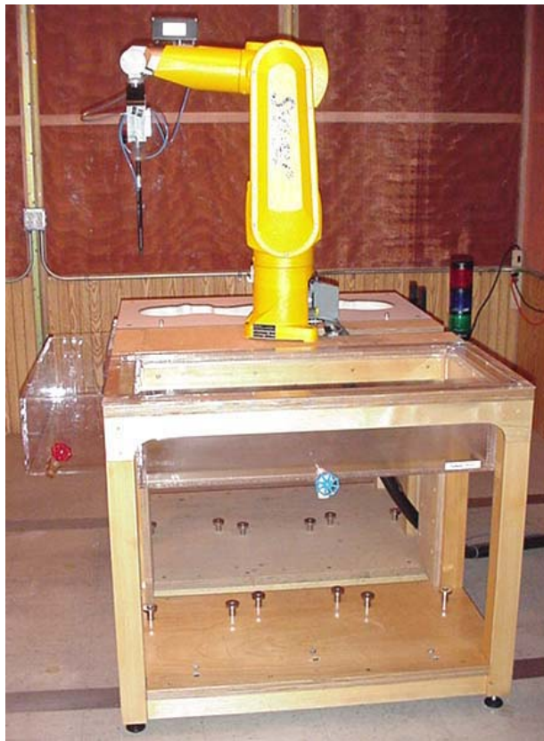
DASY4 SAR Measurement System with validation phantom
