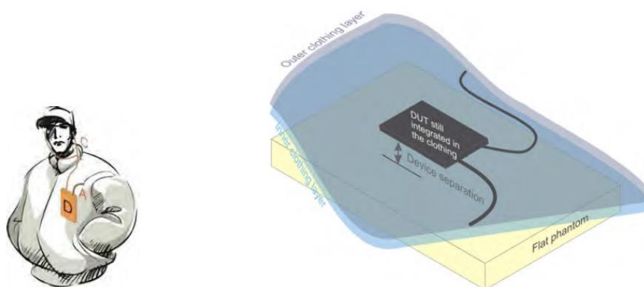
Figure 10– Test position for clothing-integrated wireless devices
