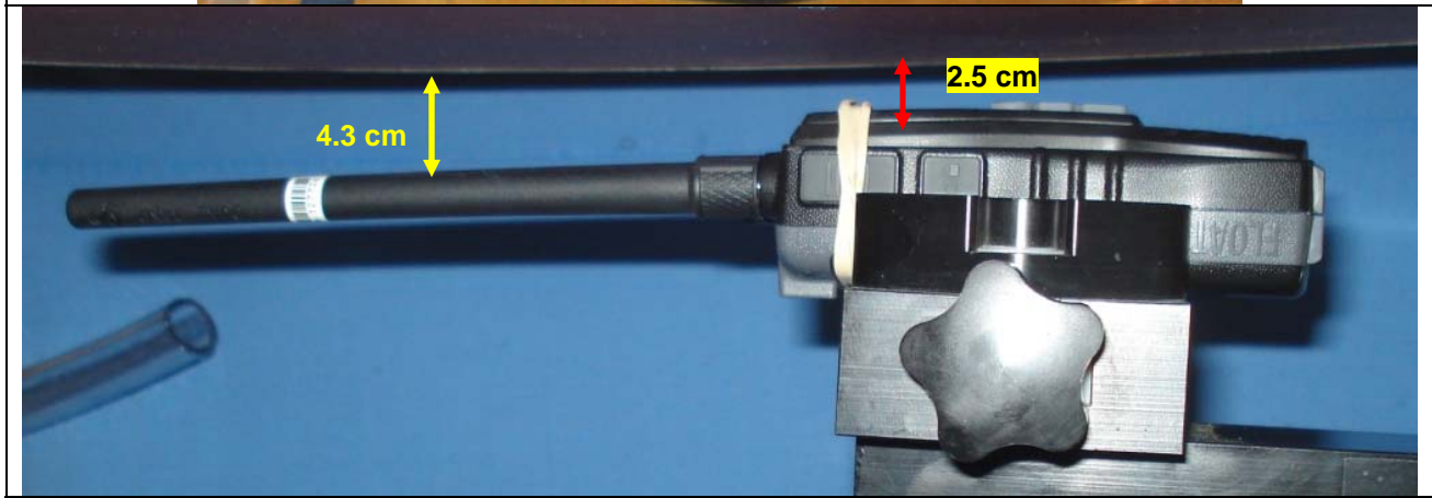
Face-held Test Setup with ELI Phantom
