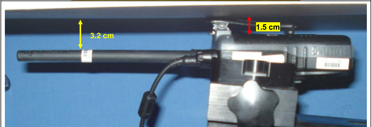
Body-worn Test Setup with ELI Phantom
