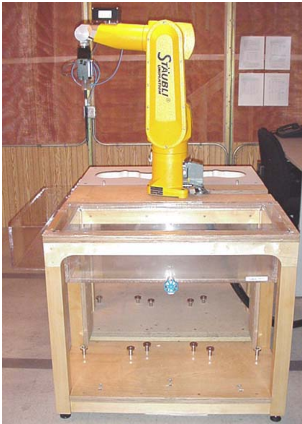
DASY4 SAR Measurement System with validation phantom
