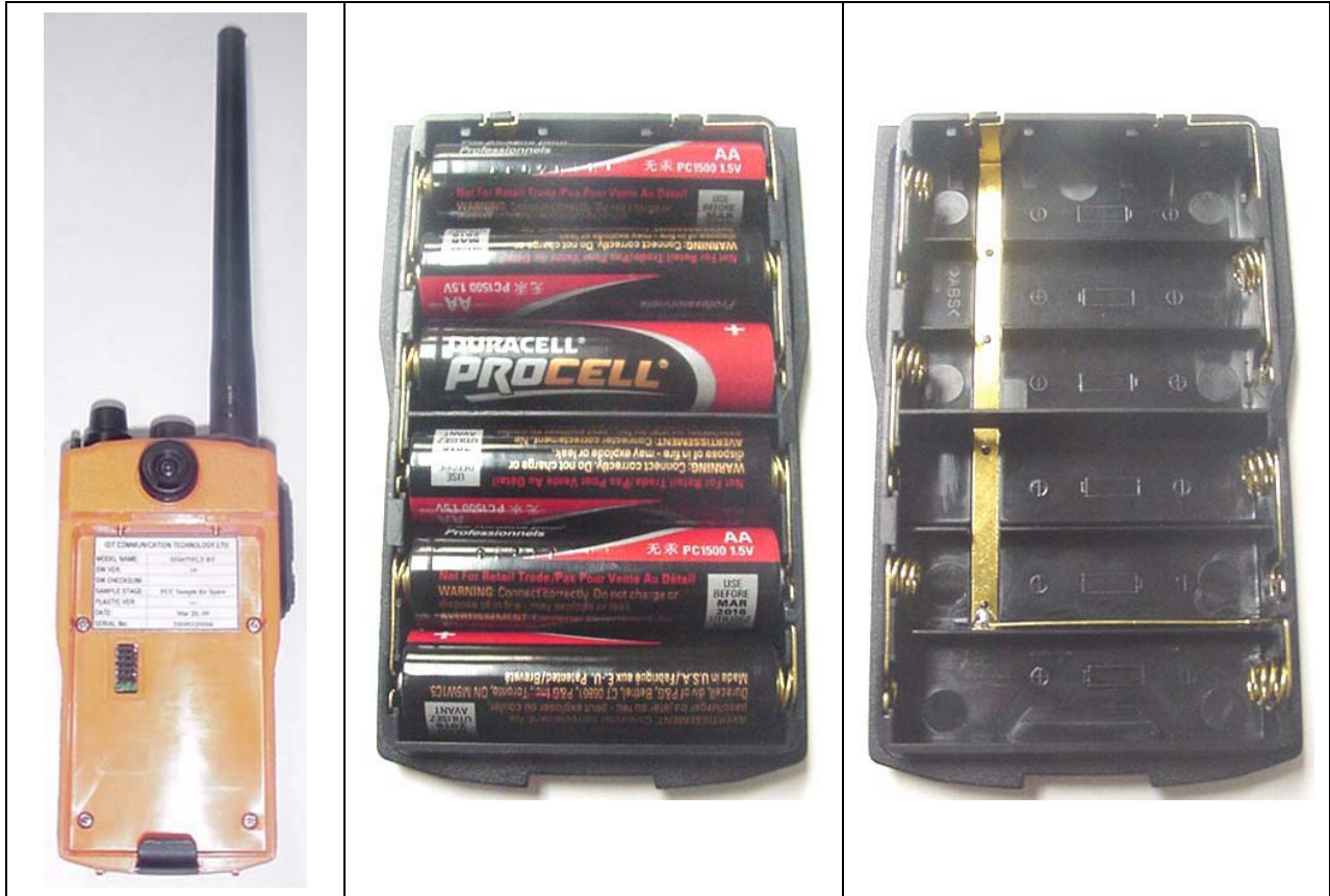
MR HH475 Battery Removed Duracell Procell Alkaline AA Batteries (x6) Alkaline Battery Tray P/N: 110-011
