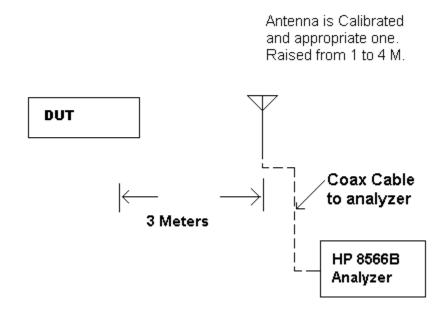
METHOD OF MEASUREMENT: The procedure used was ANSI C63.4-2003 & FCC/OET Guidance on Measurements for Spread Spectrum Systems – Public Notice DA 00-705 dated March 30<sup>th</sup>, 2000.
