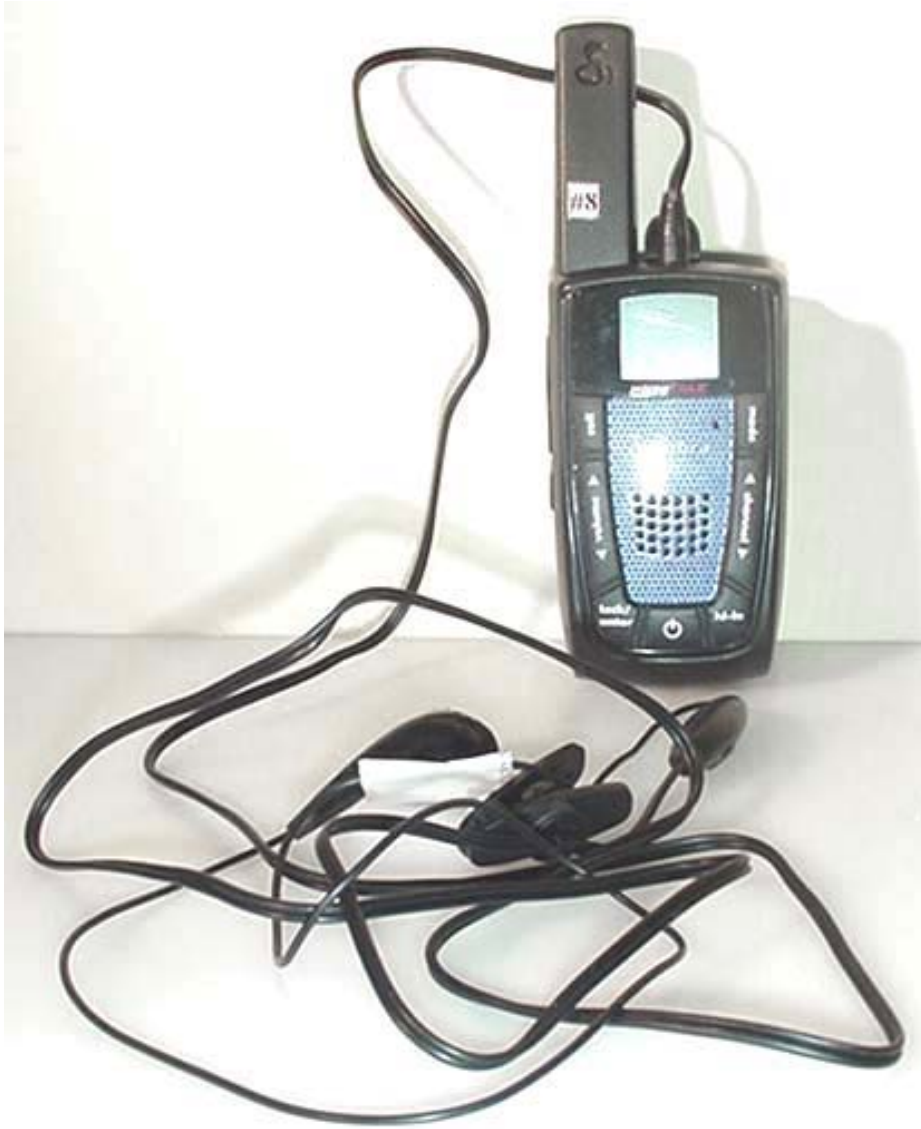
DUT with Ear-bud/Lapel-Microphone Audio Accessory
