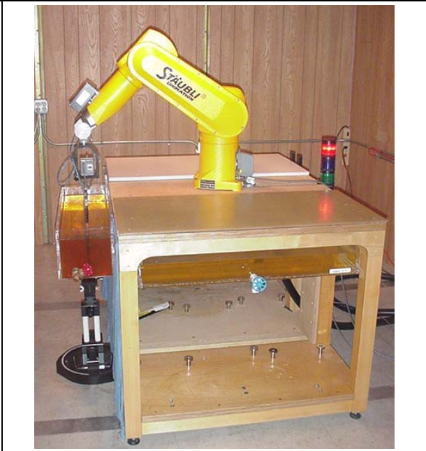
DASY4 SAR System with Plexiglas side planar phantom
