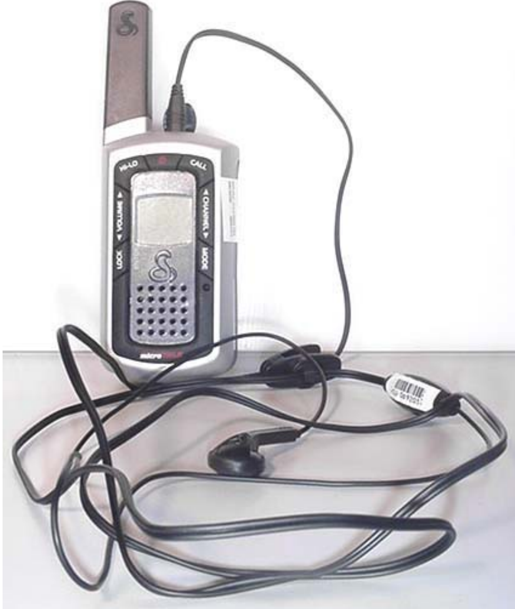
DUT with Generic Earbud & Lapel-Microphone Audio Accessory
