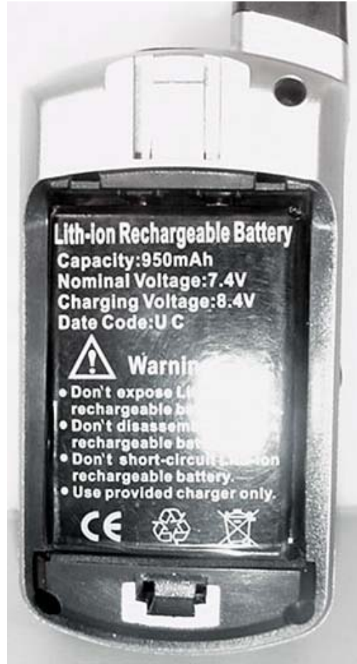
DUT with Lithium-ion Battery Pack
