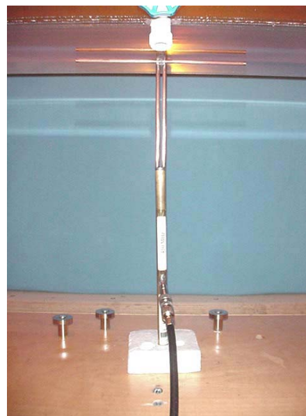
450 MHz Dipole Setup
