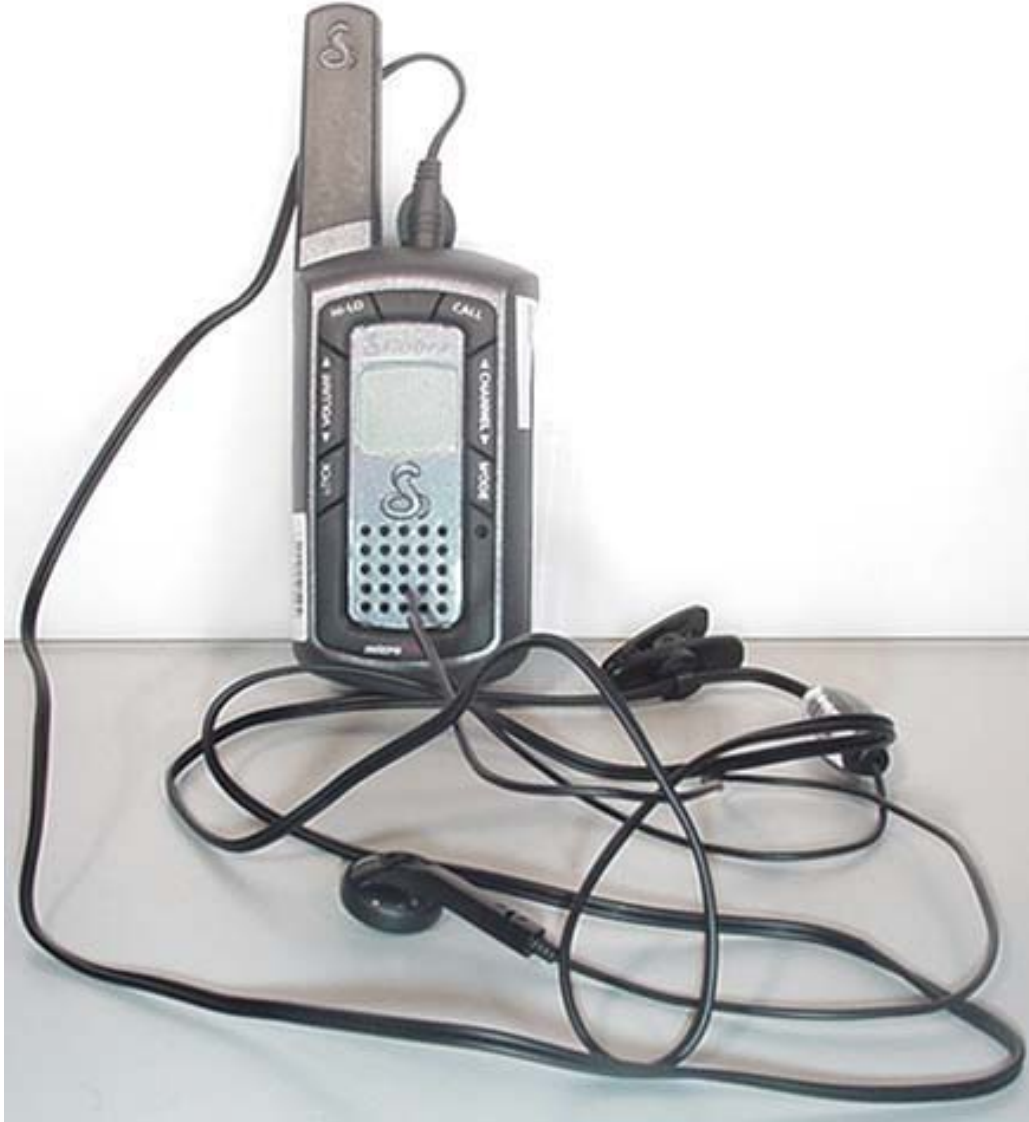
DUT with Generic Earbud & Lapel-Microphone Audio Accessory
