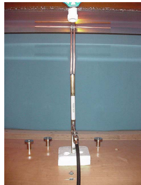
450 MHz Dipole Setup
