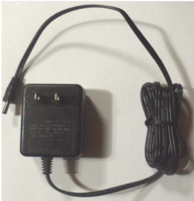
Charging Power Supply
