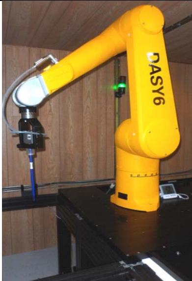
DASY 6 SAR System with SAM Phantom
