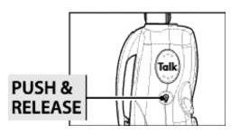
• Push and release • LIGHT/MAX RANGE button to illuminate display for ten seconds.
