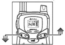
2 Select any of the 14 channels by pushing the channel up or down buttons.
