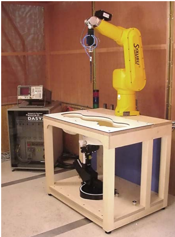
DASY3 SAR Measurement System with SAM Phantom
