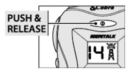
1 Push and release the OPOWER button. An audible "tone" will indicate the unit is on.
