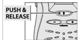
Push and release \ LIGHT/MAX RANGE button to allow all signals to enter.
