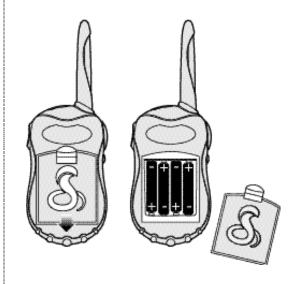
1 Pull lock tab down to remove battery cover.
