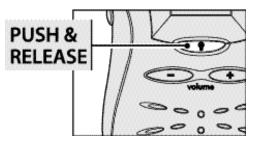
Push and release \tag{\tag{\tag{V}}} LIGHT/MAX RANGE button to illuminate display for ten seconds.
