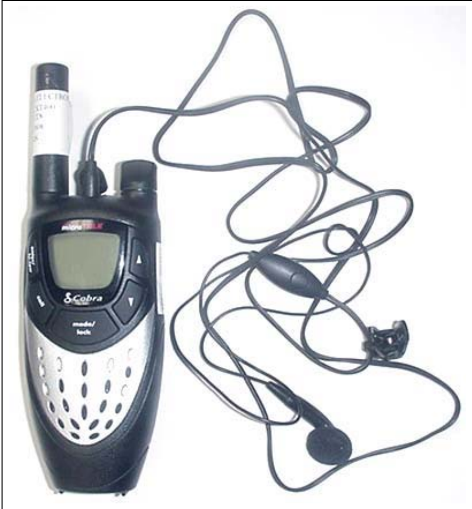
DUT with Ear-bud/Lapel-Microphone Audio Accessory (P/N: GA-EBM2)
