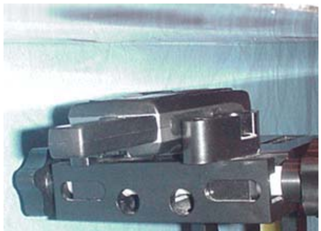
Spacing from Front of DUT to Planar Phantom = 2.5 cm
