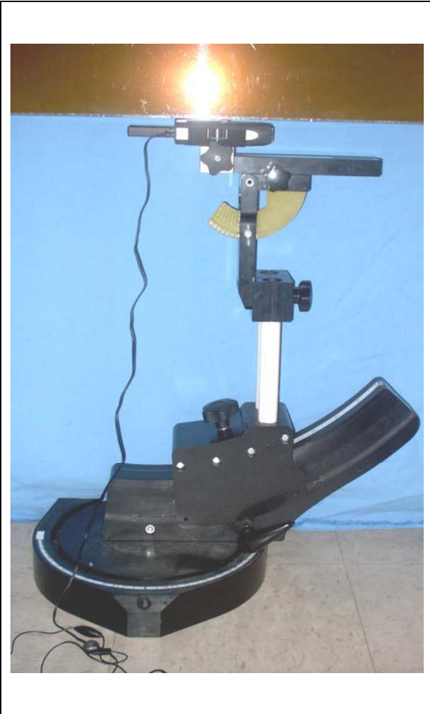
Antenna Distance to Planar Phantom = 1.1 cm
