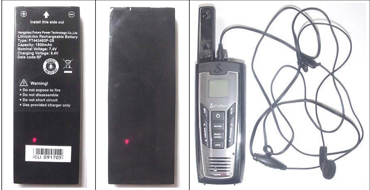
7.4V 1500mAh Lithium-ion Battery DUT with earbud/lapel-microphone audio accessory
