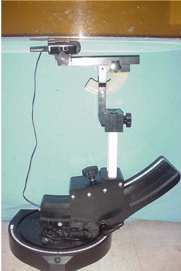
Antenna Distance to Planar Phantom = 1.5 cm
