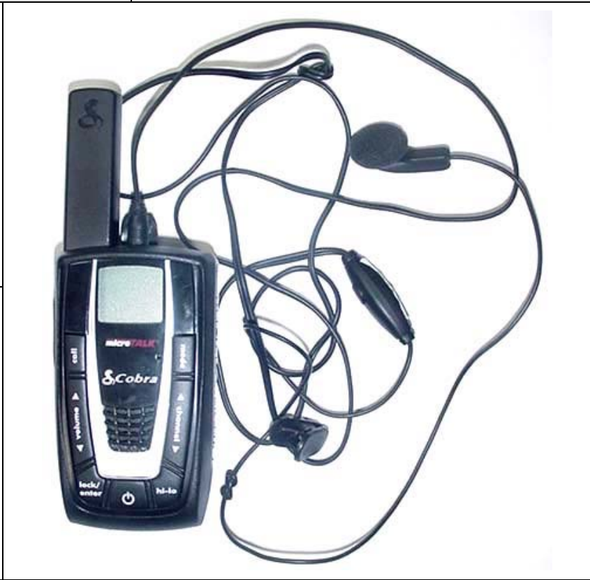
DUT with earbud/lapel-microphone audio accessory
