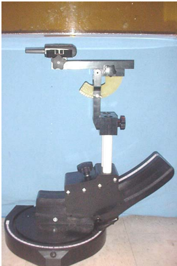
Antenna Distance to Planar Phantom = 3.4 cm
