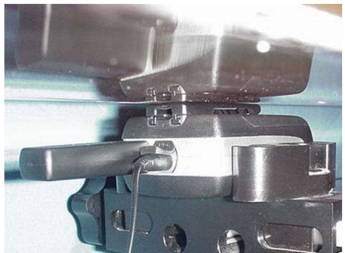
Belt-Clip Spacing from Back of DUT to Planar Phantom = 0.5 cm
