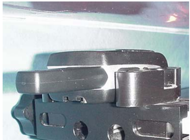
Spacing from Front of DUT to Planar Phantom = 2.5 cm
