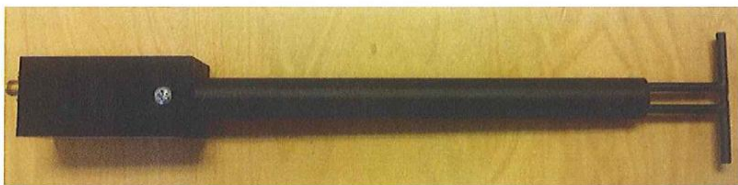
Figure 1 – MVG COMOSAR Validation Dipole
