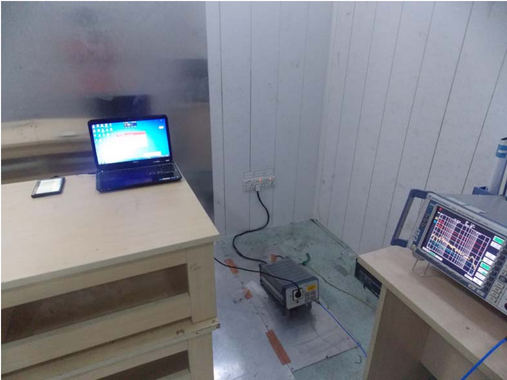
FCC RADIATED EMISSION TEST SETUP
