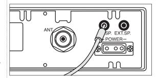
• Connect an external PA speaker to the PA jack on the rear panel.
