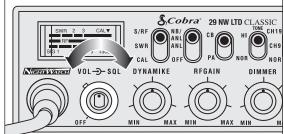
3 To achieve the Desired Squelch Setting (DSS), turn the Squelch control (a) counterclockwise until you hear noise. Now turn the control clockwise just until the noise stops. This is the DSS setting.
