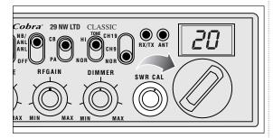
4 While holding mic button *adjust* the 🔘 SWR CAL knob so the meter needle swings to the CAL ▼ mark on the meter (located on the right).
