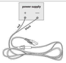
1 Simply connect the red (+) and black (-) leads of the transceiver to the corresponding terminals of the power supply.
