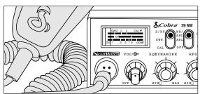
Attach the 4-pin microphone cable to receptacle on front of unit and Install unit in bracket securely.
