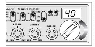
• Select One of forty channels and adjust volume. The selected channel is indicated by the LED readout directly above the channel selector knob
