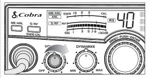
• Rotate the On/Off Volume knob clockwise. While receiving, the RX icon will be displayed and the lower portion of the meter will show the incoming signal strength.
