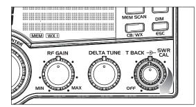
4 While holding the PTT adjust the **SWR CAL** knob so the meter swings to the CAL mark on the right side of the meter.
