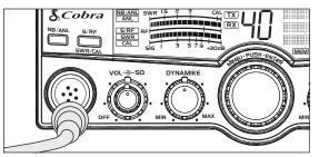
Attach the microphone cable to the receptacle on the front of the unit and install the unit in the bracket securely.
