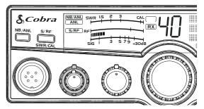
To achieve the Desired Squelch Setting (DSS), rotate the **Squelch** knob *counterclockwise* until you hear noise. Now rotate the knob *clockwise* just until the noise stops. This is the DSS setting.
