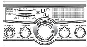
• Rotate the **Channel Selector** *clockwise* or *counter-clockwise* to select the desired channel.
