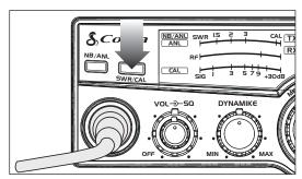
Press S/RF-SWR/CAL button to select CAL.
