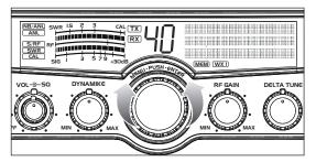
3 Select one of forty channels. The selected channel (1 through 40) will be indicated by the readout directly above the channel selector knob
