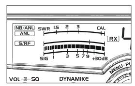
• The S/RF-SWR/CAL button must be set in the S/RF setting to read the meter.
