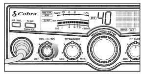
2 Full counterclockwise rotation opens the "gate" allowing all signals in.
