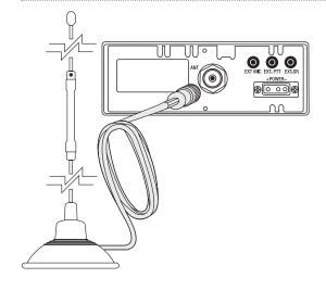
**3** Connect the antenna cable plug to the receptacle marked "ANT" on the back of the unit.
