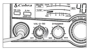
1 Rotate the **On/Off Volume** knob *clockwise* to turn the unit on and adjust to a normal listening level.
