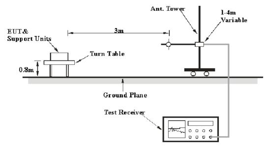
The radiated emissions were performed in the 3 meters distance, using the setup accordance with the ANSI C63.26-2015. The specification used was the FCC Part 95 limits.
