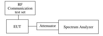
Note: the path loss(cable loss and attenuator) has included into the plot.
