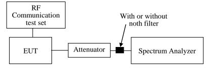
Note: the path loss(cable loss and attenuator) has included into the plot.
