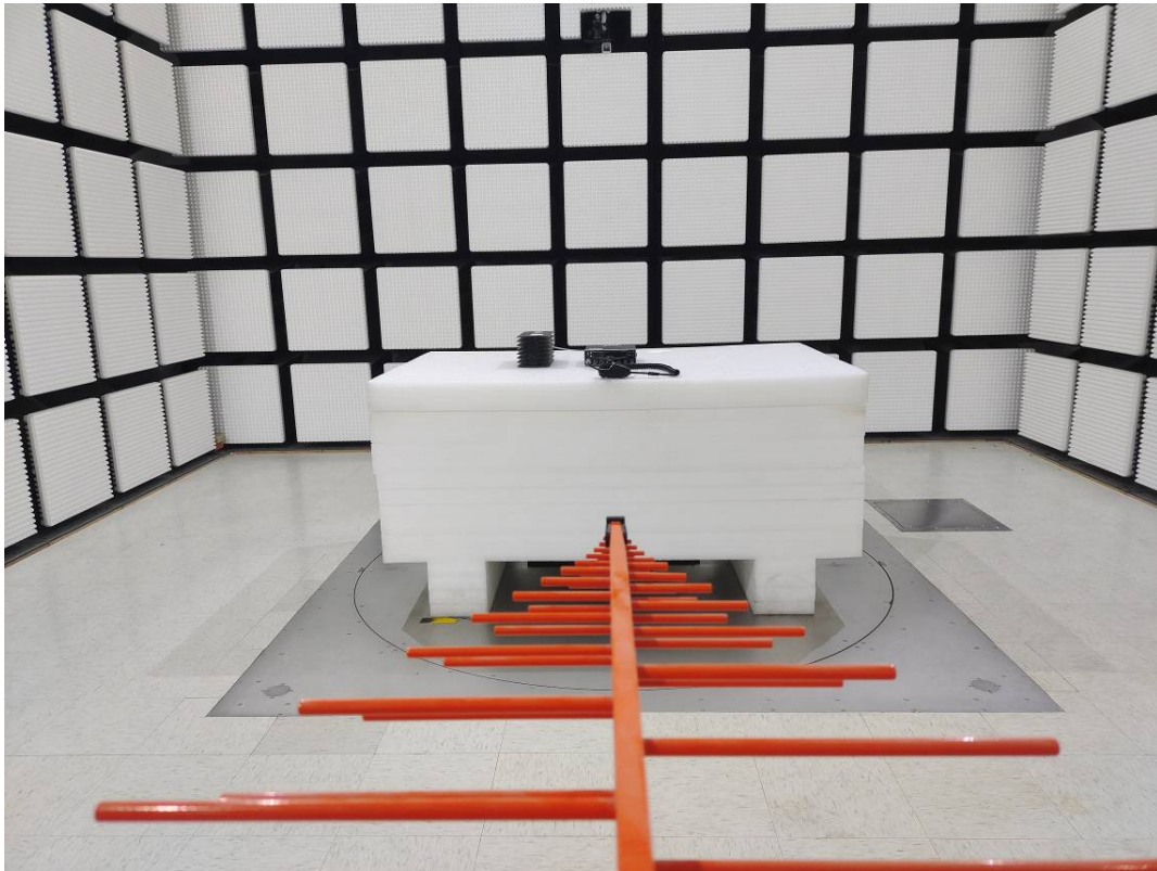
Radiated Emission Below 1GHz View
