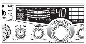
Select one of forty channels and adjust volume. The selected channel (1 through 40) will be indicated by the readout directly above the channel selector knob
