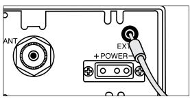
• Connect an external speaker to the external speaker jack on the rear panel.
