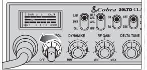
2 Full @ counterclockwise rotation opens the "gate" allowing all signals in.
