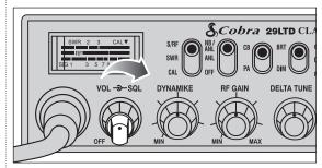
2 Rotate the On/Off Volume knob clockwise to a normal listening level.
