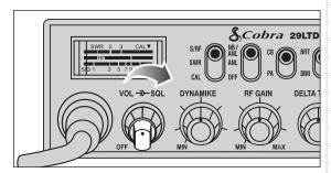
Rotate the On/Off Volume knob *clockwise*.
