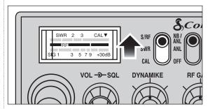
The S/RF-SWR-CAL switch must be in the S/RF position.
