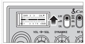
**1** The S/RF-SWR-CAL switch must be in the S/RF position to read the meter.
