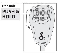
• Push and hold the mic button to transmit. The transmitter is now activated. When transmitting, hold the microphone two inches from your mouth and speak in a clear, normal voice. Release to receive.
