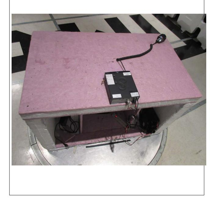
Radiated Tests Above 1 GHz: In Band Field Strength/ Restricted Band Emissions
