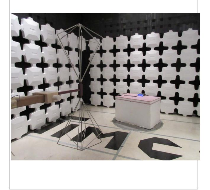
Radiated Test Below 30 MHz: Restricted Band Emissions
