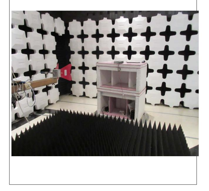
Radiated Test Below 1 GHz: Restricted Band Emissions
