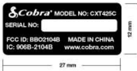
CXT425 / CXT475 SERIAL NUMBER LABEL BLACK LABEL, SILVER TYPE, HELVETICA BOLD FONT 200%
