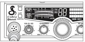
8 Attach the microphone cable to receptacle on front of unit and install unit in bracket securely.
