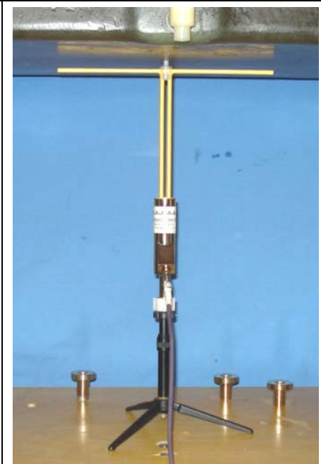
SPEAG 450 MHz Validation Dipole Setup
