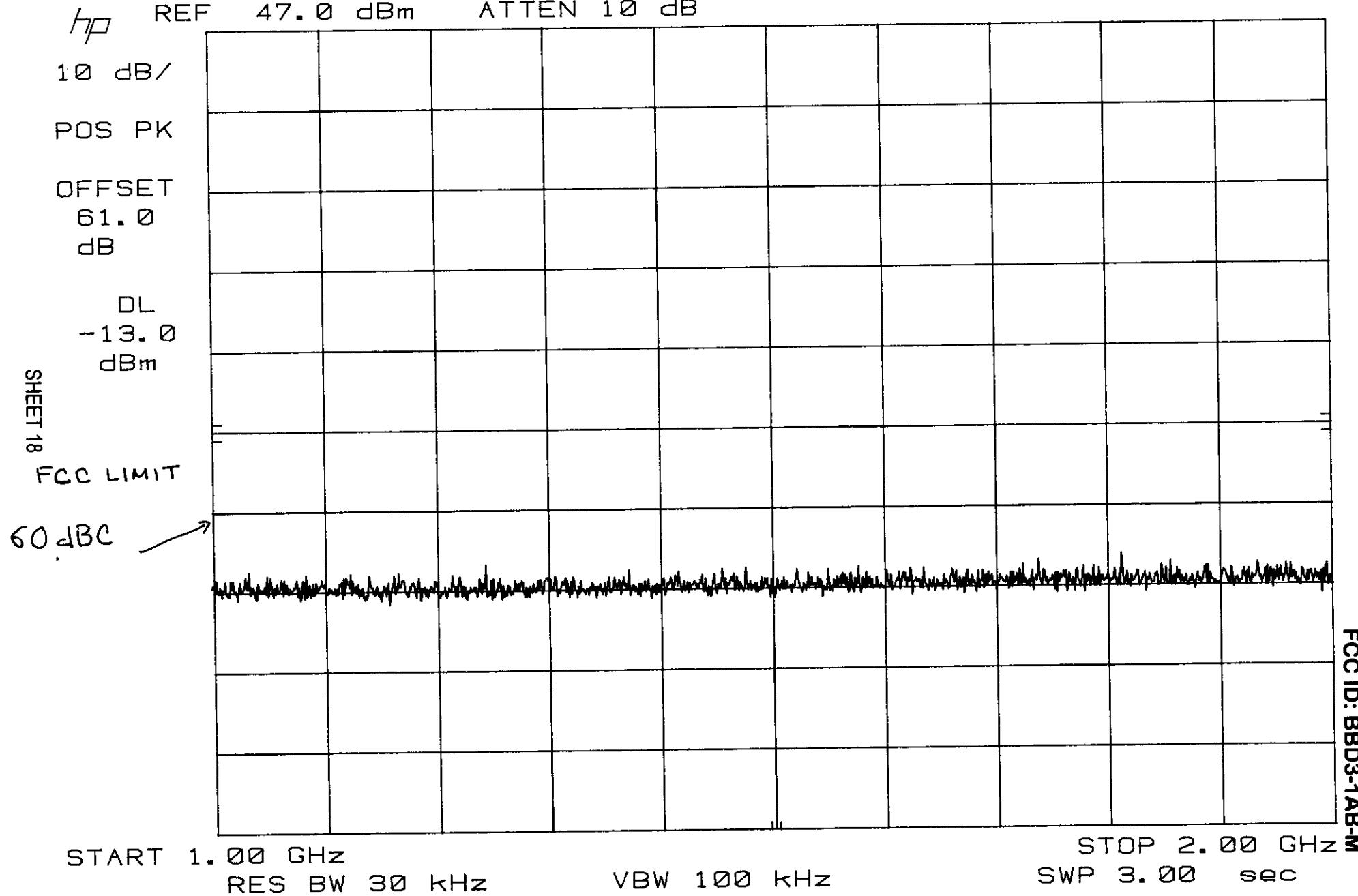
**2.983(e)(5) Measurement of Radiated Spurious Emissions per 2.993****Definition:**
