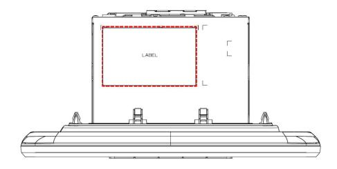
The label material is Yupo 80 (UV) and the ink is UV ink, which has improved durability against repeated rubbing tests compared to ordnary synthetic paper.
