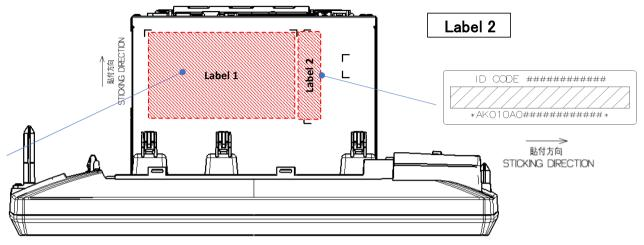
The label material is Yupo 80 (UV) and the ink is UV ink, which has improved durability against repeated rubbing tests compared to ordinary synthetic paper.
