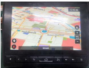
By pressing this button, the direction of the map is toggled as follows: North Up  $\to$  Heading Up  $\to$  3D Heading Up
