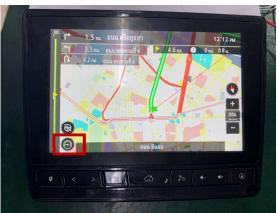
Press the red frame part of the screen, and the navigation sound will come out manually.
