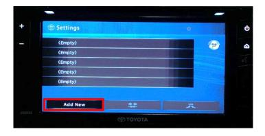
6 Turn on the Bluetooth function of the device to be paired and connect to the radio unit.
