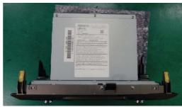
When the panel and the front plate are dismounted.
