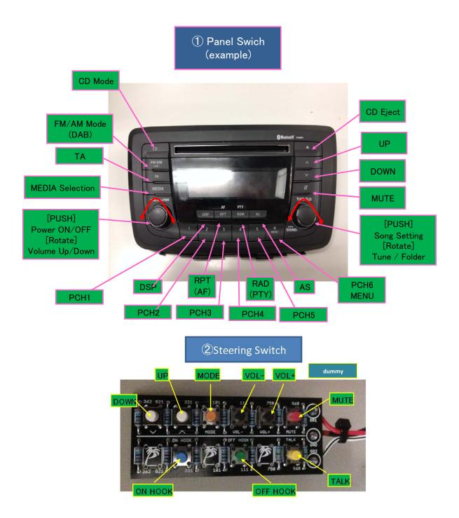
Bluetooth Setup: press "TALK" button on steering switch
