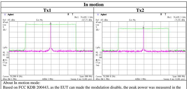
Based on FCC KDB 200443, as the EUT can made the modulation disable, the peak power was measured in the non-modulation mode.
