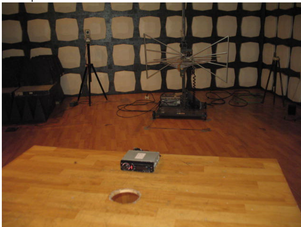
Radiated Emission Test Set-Up
