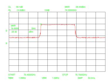
The occupied frequency is between 76.500 GHz and 76.605 GHz
