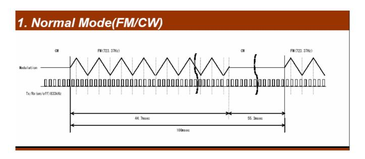
As the output is switched on/off with 50% duty cycle, we have a correction factor of -3 dB.
